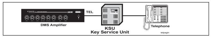
Fig. 13 - Connecting to the Telephone Paging KSU
